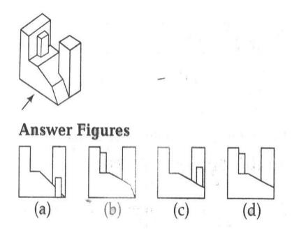
33. The 3-D problem figure shows an object. Identify the correct front view, from amongst the answer figures, looking in the direction of arrow?
